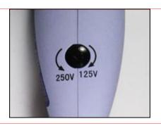
In this final image, you can see that some appliances have a switch for use between higher and lower voltages. This can be used overseas with only a **plug adaptor**, but do not forget to flip the switch!
