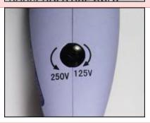
In this final image, you can see that some appliances have a switch for use between higher and lower voltages. This can be used overseas with only a **plug adaptor**, but do not forget to flip the switch!
